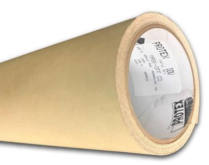
**PROTEX 10V** is a 10 mil latex saturated paper, which has a vinyl coating on one side to increase its abrasion resistance. It can be used in the protection of acrylic and polycarbonate windows, canopies and windshields. It can also be used for bare metal and painted surface protection where added abrasion resistance is required. A liner allows the product to be die-cut if desired.
